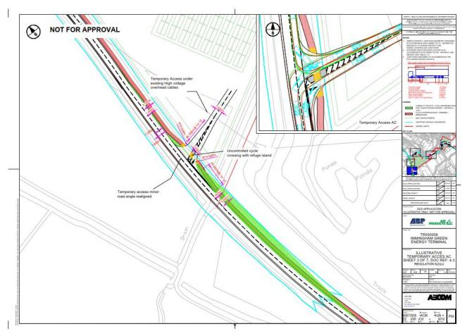
3.1.6 As can be seen in **Plate** 8, Temporary Access AC is a simple priority junction from the A1173 and has been designed to accommodate max legal HGV movements.
