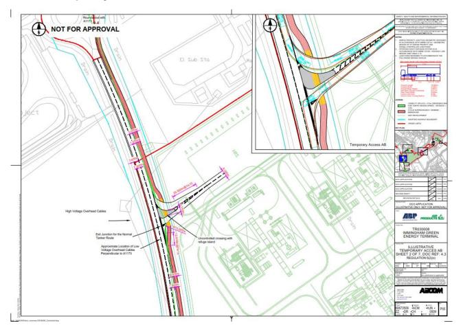
3.1.5 As can be seen in Plate 7, Temporary Access AB is a simple priority junction from the A1173 and has been designed to accommodate max legal HGV movements.
